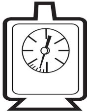
**Oven Thermometers:** An oven thermometer can be left in the oven to verify that the oven is heating to the desired temperatures. These bimetallic-coil thermometers can measure temperatures from 100 °F to 600 °F.
