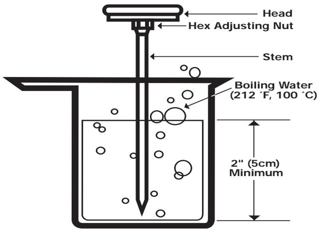
For true accuracy, distilled water must be used and the atmospheric pressure must be one atmosphere (29.921 inches of mercury). A consumer using tap water in unknown atmospheric conditions would probably not measure water boiling at 212 °F. Most likely it would boil at least 2 °F and perhaps as much as 5 °F lower. And, remember that water boils at a lower temperature in a high altitude area.
